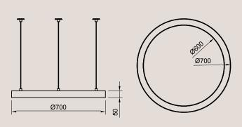
**Please note:** the electrical cable runs up one of the end hanging support wires and is encased in a clear plastic sleeve.
