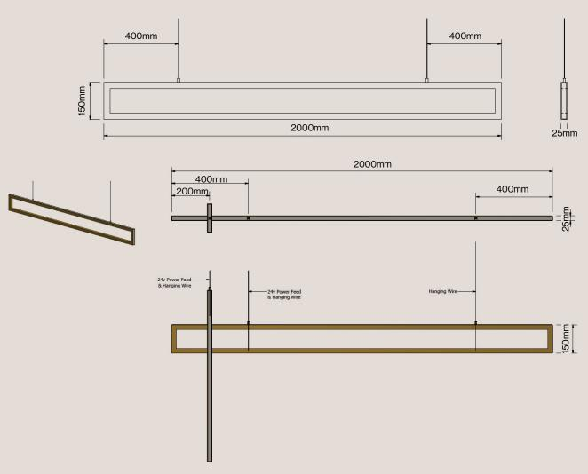
Wire Specifications (for 600 L x 150 H x 25 D vertical Elevation Pendant) Standard length of hanging support wire is 3m. Standard length of hanging electrical wire is 4m.
