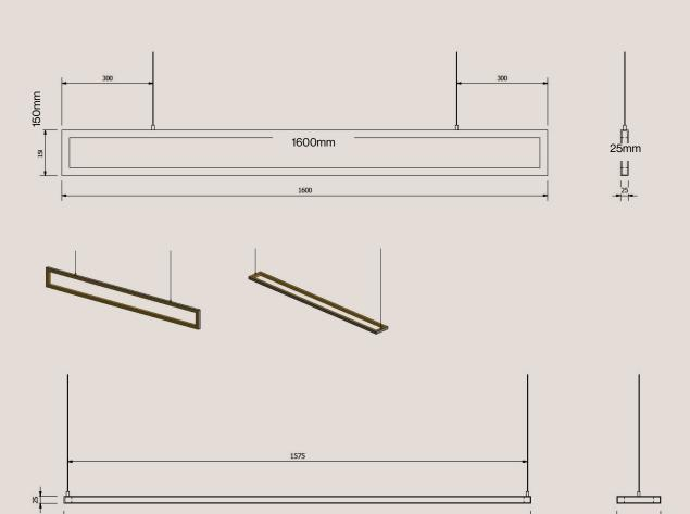
Wire Specifications (for 2000 L x 150 H x 25 D horizonatal Elevation Pendant) Standard length of hanging support wire is 1.8m. Standard length of hanging electrical wireis 3m. This will be long enough to suit a floor-to-ceiling (stud) height at a max of 3.6 metres.
