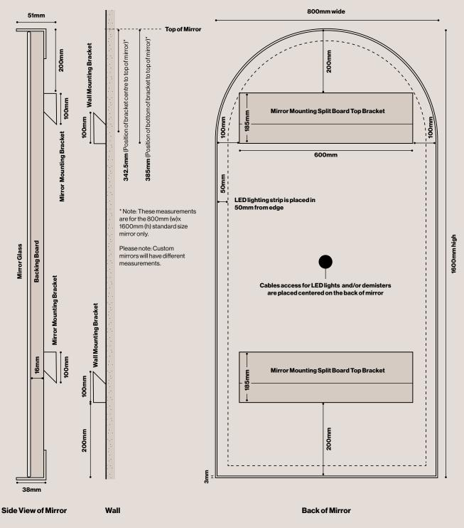
Note: Demister cable is white Demister model: Nu-klear 230v **Note:** LED cable is clear (white stripe = postive) **LED transformer:** 24v 800w
