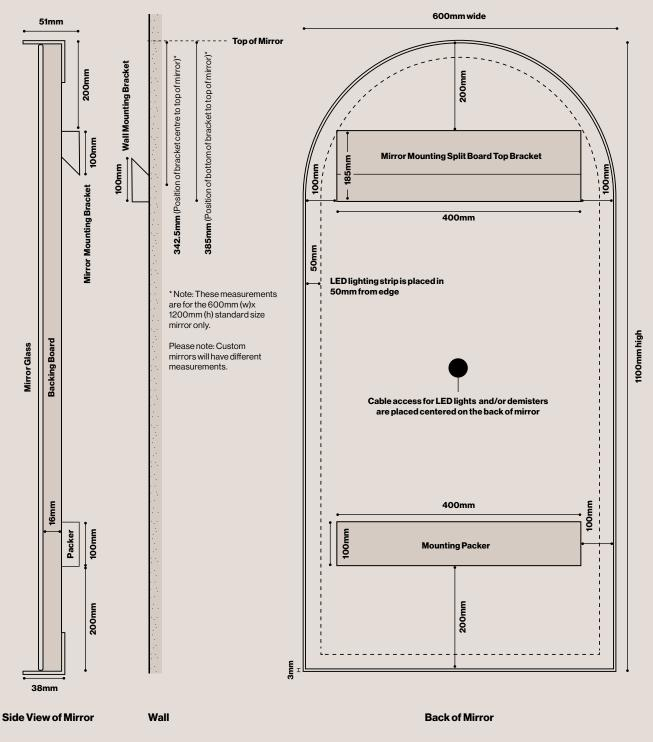
Note: Demister cable is white Demister model: Nu-klear 230v Note: LED cable is clear (white stripe = postive) LED transformer: 24v 80w
