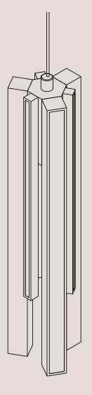
**Please note:** the electrical cable runs up one of the end hanging support wires and is encased in a clear plastic sleeve.
