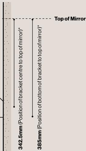
\* Note: These measurements are for the 600mm (w) x 1200mm (h) standard size mirror only.
