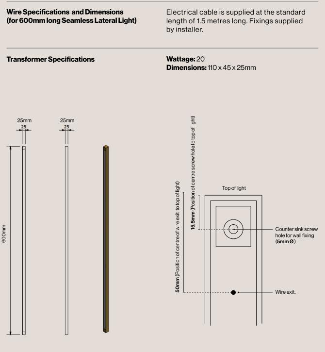
**Close-up of wall fixing postion** Please note: the bottom of the light has the matching wall fixing position)
